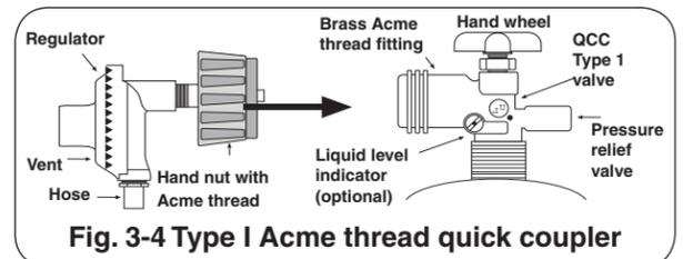
Fig. 3-4 Type I Acme thread quick coupler
