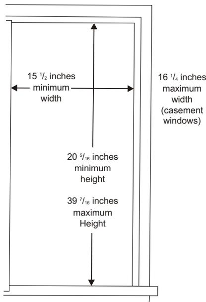
**NOTE:** Height measurement must be of a clear opening above mounting platform. In some cases, due to a variety of stop and track arrangements, the above dimensions may vary slightly. If necessary, installation can be made by alternating window jambs. (See Alternate Window Jamb Applications.)
