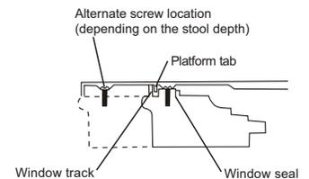
**Center platform assembly on the line with platform tab pressed against window track**
