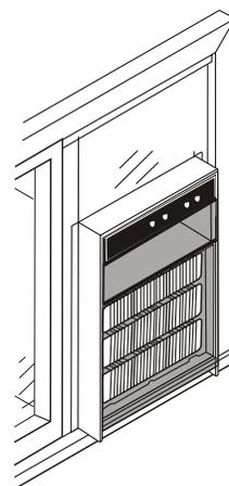
**14. Drill two 9/64-inch diameter pilot holes** in the top window jamb in line with the partially plugged holes in the panel frame. Secure the panel frame to the window jamb with two #8-32x3/4-inch self-threading screws. If additional holding is necessary, two screws may be used on the sides of the panel frame as well.
