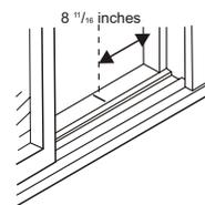
Apply track seal to the outside edge of the bottom window jamb.
