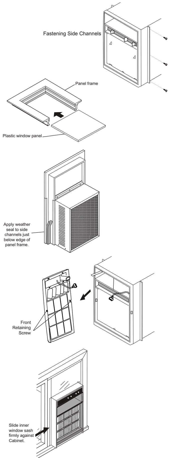
**16. Slide inner window sash firmly** against side of the cabinet. Make sure not to peel the seal strips from the window track and cabinet side channels. If the panel frame does not fit snugly to the inner window sash, secure the panel frame to the sash with #8x3/4-inch screws, or #8-32x3/4-inch self-threading screws. Use the partially plugged holes in the panel frame. Drill 1/8-inch pilot holes for the screws.
